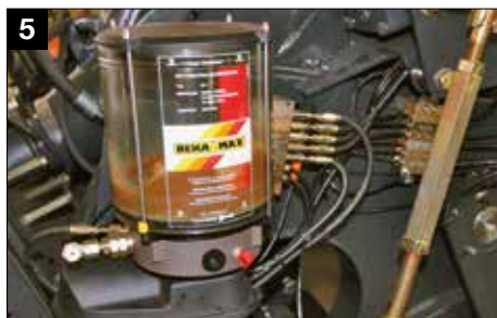
5 Automatic greasing system
