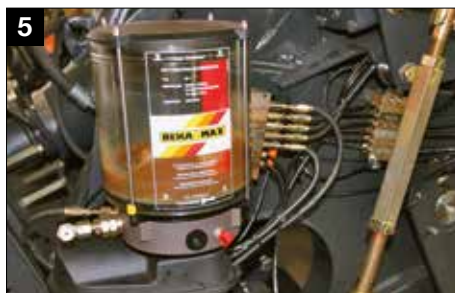
5 Automatic greasing system
