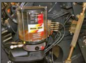
Automatic greasing system
