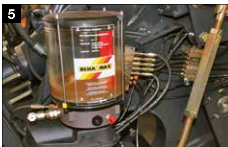
Automatic greasing system
