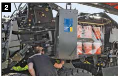
Pivoting twine boxes for easy maintenance
