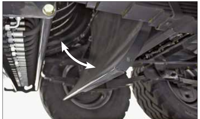
Pre-chamber inspection door
