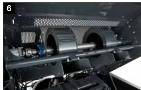
6 Knotter cleaning turbines
