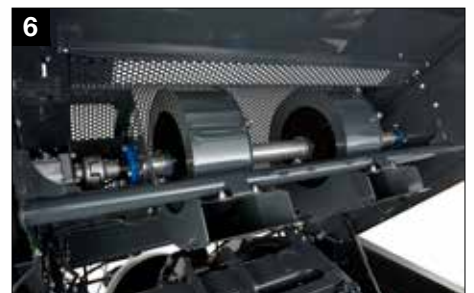
6 Knotter cleaning turbines
