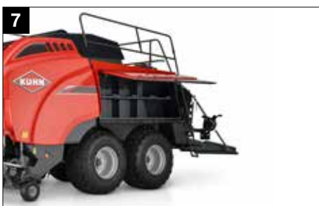
Easy accessible twine boxes with 2x16 capacity
