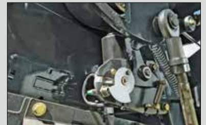
Electric binding system
