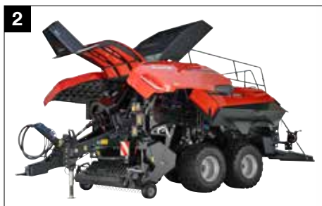
2 Pivoting twine boxes for easy maintenance
