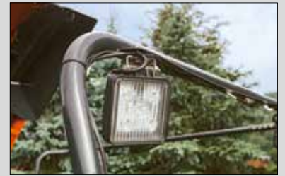
LED working lights
