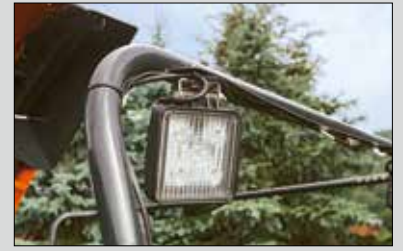
LED working lights
