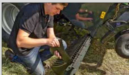
One-sided sliding knife cassette system
